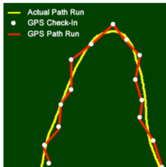
The image to the right shows what happens 95% of the time. So the result is that your GPS can read your path as weaving 10 meters in either direction, when you are actually moving in a straight line.
